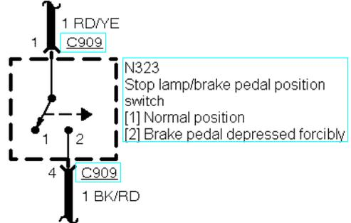
ABS with Traction Control System (TCS)
